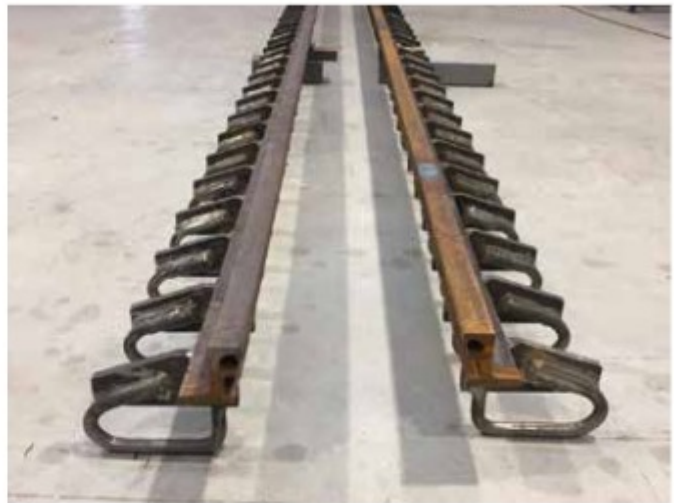
Fabrication of AR-EX HS—Before Painting
